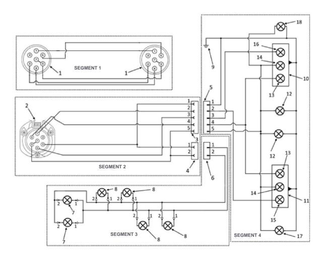
Figure 12. A diagram of the Trailer's electric system (version with side position lamps):
