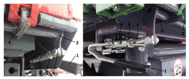
The locks on the sideboards of the load-carrying body: 1 - bottom locks lever, 2 - locks central roller, 3 - locks, 4 - turnbuckle, 5 - counter-nut, 6 - threaded connector
