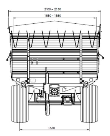
Figure 8. Dimensions of the Trailer – front view
