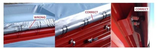
Figure 3. Correct tensioning of the tarpaulin cover
