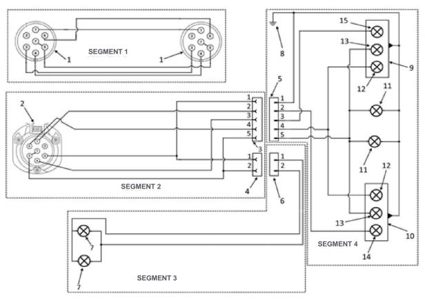
A diagram of the Trailer's electric system (basic version): 1 - 7-pole plug, 2 - 7-pole socket, 3 - 5-PIN superseal female plug, 4 - 2-PIN superseal female plug, 5 - 5-PIN superseal male plug, 6 - 2-PIN superseal male plug, 7 - front position light bulb, 8 - ground, 9 - 3-way right rear lamp, 10 - 3-way left rear lamp, 11 registration plate lamp bulb, 12 - STOP lamp bulb, 13 - rear position lamp bulb, 14 left direction indicator lamp bulb, 15 - right direction indicator lamp bulb
