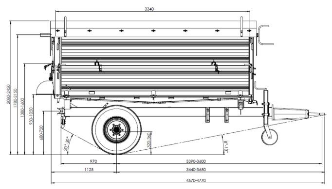
Figure 9. Dimensions of the Trailer – side view
