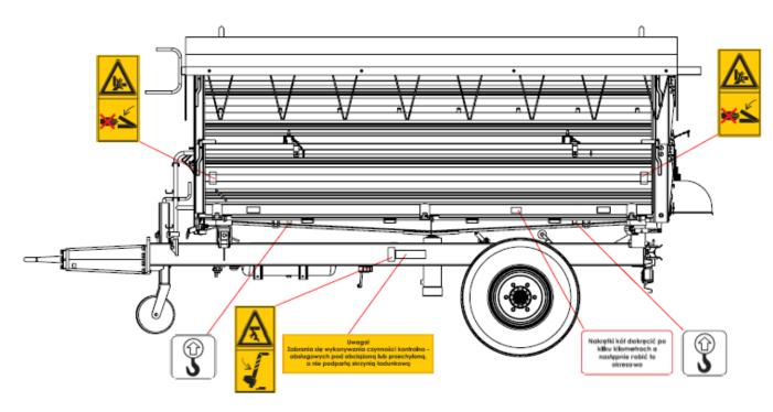
Figure 7. The arrangement of the pictograms on the boards of the Trailer – left side
