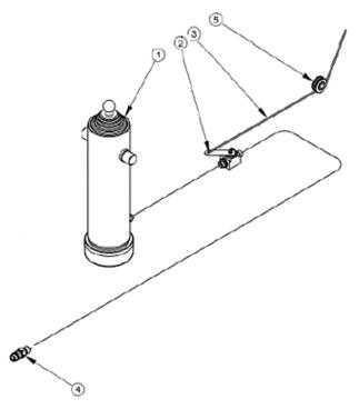
The diagram of the hydraulic system in the tilting mechanism of the Figure 10. Trailer's body:
