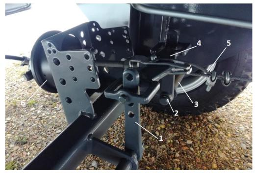
Figure 17. The components of the brake system: 1 - expander roller lever, 2 - adjusting nut, 3 - expander roller, 4 - brake equalising bar, 5 - parking brake cable, 6 - cylinder
