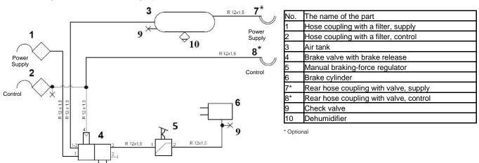
Figure 13.A diagram of a dual-line pneumatic braking system
