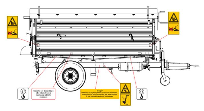
Figure 6. The arrangement of the pictograms on the boards of the Trailer – right side
